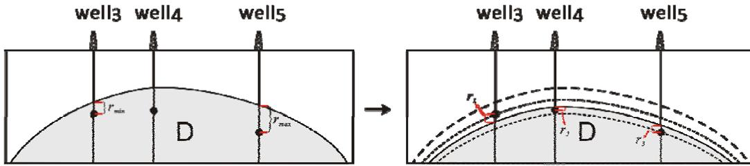
**Figure 9:** Schematic diagram illustrating the well conditioning methodology with multiple wells case. The minimum and maximum residuals are calculated first, i.e.,  $r_{min}$  and  $r_{max}$  on the left plot; then the candidate surface is “lower” down in-between the minimum and maximum residual; after that, the residual of each available well pick to the new surface,  $r_1$ ,  $r_2$ , and  $r_3$ , are calculated (the right plot).
