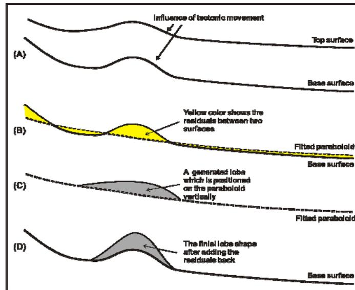
**Figure 3:** a diagram illustrating that the paraboloid and incline base surface transform may reproduce the influence of tectonic movements.
