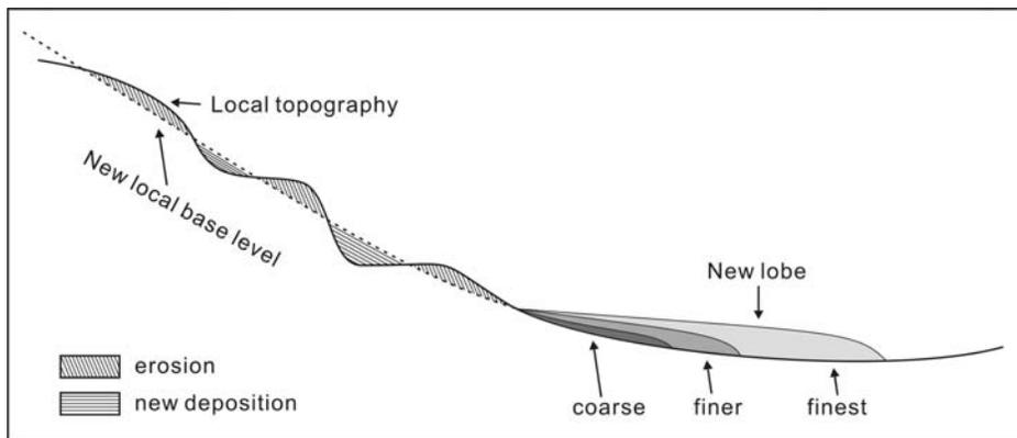
**Figure 6:** A schematic diagram showing the local base profile forming procedure. The vertical scale has been exaggerated to illustrate the local erosion and new deposition process.
