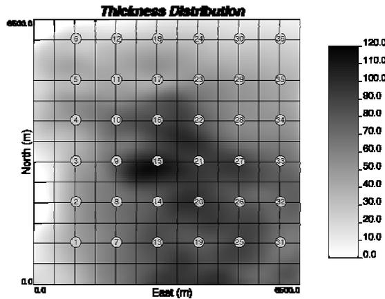
**Figure 10:** Well location map with thickness distribution map as the background. Regular well pattern is assumed and 36 synthetic wells are designed.
