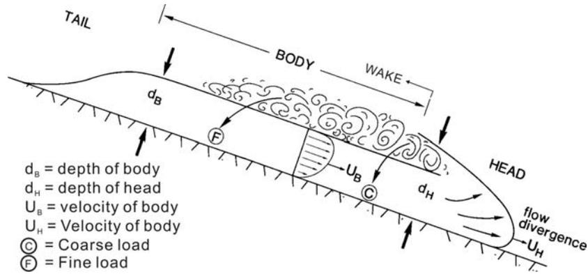
**Figure 5:** Simplified sketch of a large turbidity current, divided into head, body and tail regions. Settling from the wake behind the head produces a lateral size grading in the flow (after Pickering *et al.* 1989).
