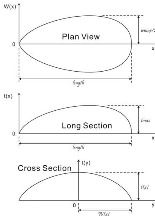
**Figure 1:** Parameters needed to describe the 3-D lobe geometry.
