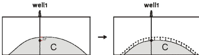
**Figure 8:** Schematic diagram illustrating the well conditioning methodology with one well case. The residual of the available well pick with the candidate surface is calculated first (left plot); then the candidate surface is “lower” down to pass through the available well pick based on the residual (right plot).
