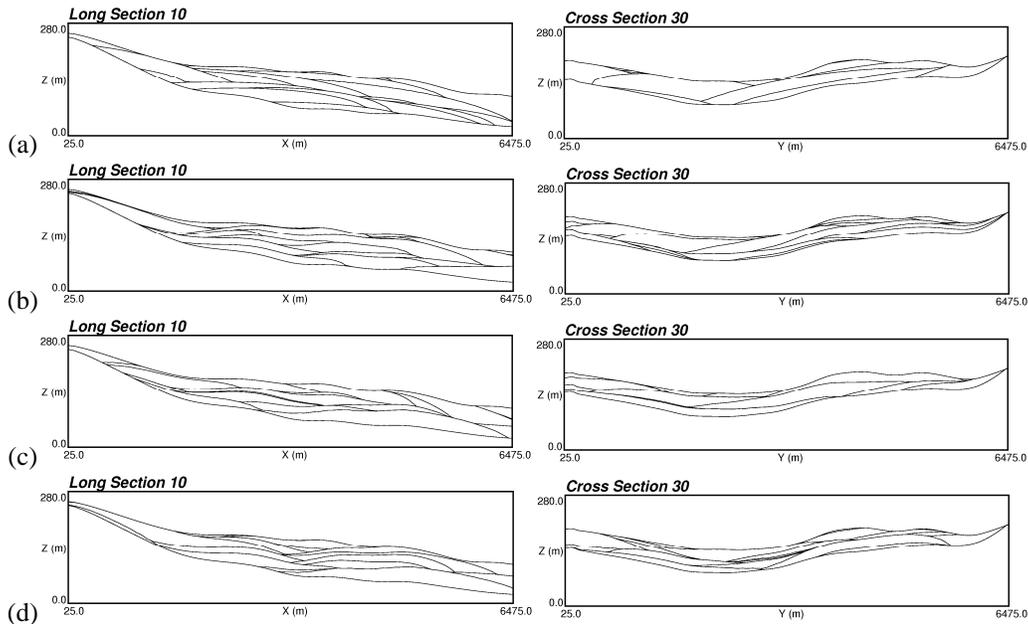
**Figure 11:** A long section and a cross section showing the unconditional simulation results with different base surface transform: (a) without base surface transform; (b) flatten base surface; (c) transform base surface to a paraboloid; and (d) transform base surface to an incline. 45, 82, 45 and 68 surfaces were generated, respectively.
